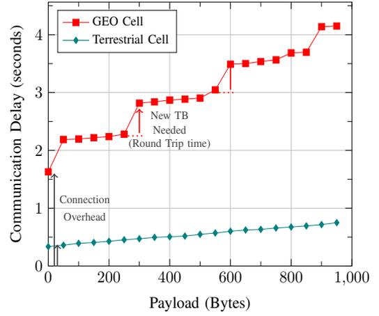
Fig. 9: Delay of communications from first connection attempt to last payload bytes sent, depending on payload and cell type. The differences are due to coverage and round trip delay. Data plotted for BLER =  $10^{-1}$ .
