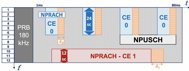
Fig. 4: Differential delay impact on UL Frame
