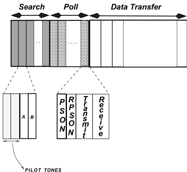
Fig. 1. Frame structure in PMAC.
