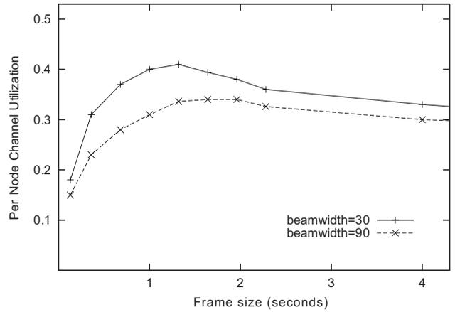
Fig. 10. Per node CUR achieved vs. frame size in random mobile topology with speed = 10m/s.
