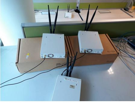
**Figure 2: USRP testbed used for implementing and evaluating diamond-based relaying.**
