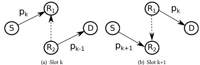
Figure 1: Two-path relaying illustration
