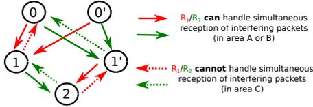
**Figure 6: Source rate adaptive protocol state machine**
