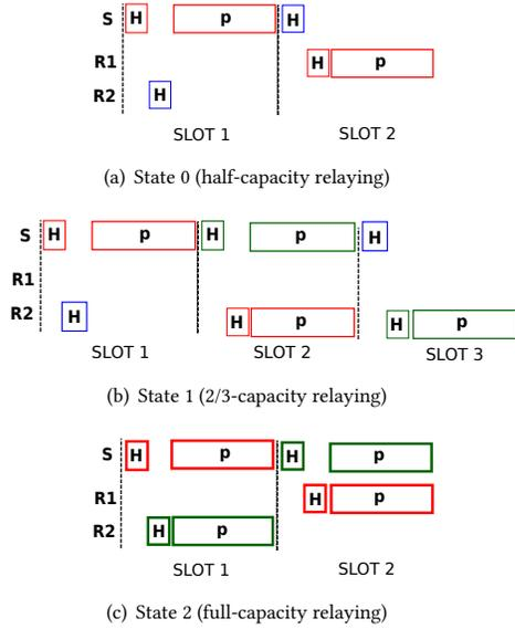
**Figure 5: COLiDeR introduces 3 scheduling policies: the traditional half-capacity one-path relaying (5(a)); 2/3-capacity two-path relaying (5(b)); and full-capacity two-path relaying (5(c)).**
