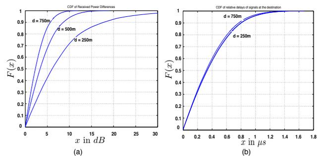
Fig. 2. CDFs of (a) the power difference and (b) relative delays
