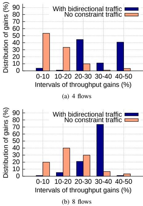
Fig. 6. Distribution of throughput gains depending on the traffic pattern for 4 and 8 established flows
