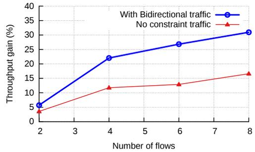
Fig. 5. Gains of TWRC PLNC in a multi-hop network depending on the traffic load
