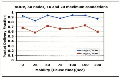
Fig. 5. Drop in the packet delivery fraction for AODV, when doubling the number of maximum connections.
