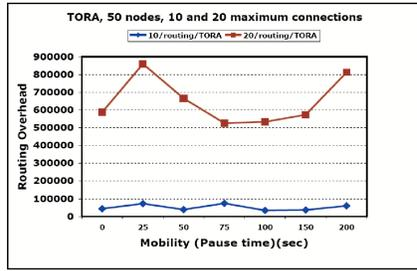
Fig. 9. Increase in routing information exchange for TORA, when doubling the number of maximum connections.
