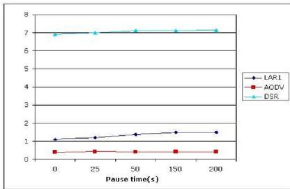
Fig. 2. Average end-to-end delay in seconds for LAR, DSR and AODV.
