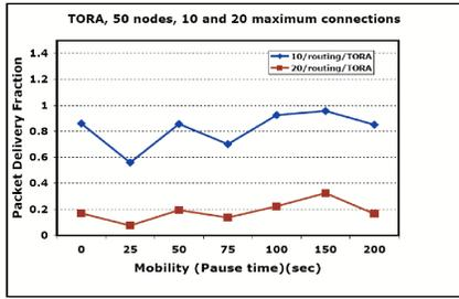
Fig. 8. Drop in the packed delivery fraction for TORA, when doubling the number of maximum connections.
