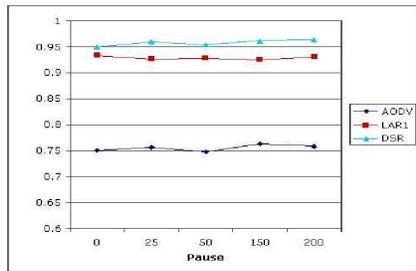
Fig. 1. Packet Delivery Fraction (PDF) for LAR, DSR and AODV.
