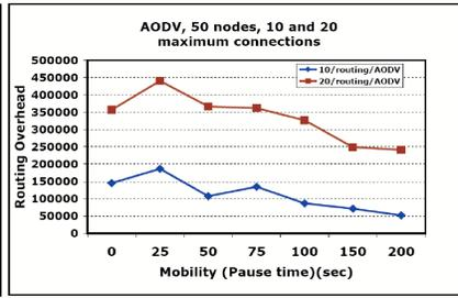
Fig. 6. Increase in routing information exchange for AODV, when doubling the number of maximum connections.
