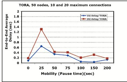
Fig. 7. Increase in the average end-to-end delay for TORA, when doubling the number of maximum connections.
