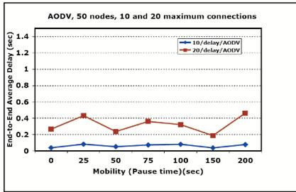
Fig. 4. Increase in the average end-to-end delay for AODV, when doubling the number of maximum connections.
