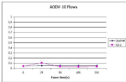
Fig. 11. Average end-to-end delay in seconds for AODV.
